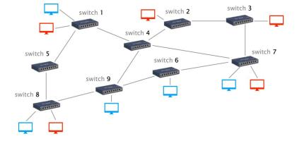
A network below consists of 9 switches and hosts in two different VLANs (blue and red).
