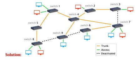
Using the previously computed spanning tree, which path will the red host connected to switch 7 use to communicate with the red host connected to switch 1?
