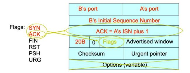
B tells A it accepts, and is ready to hear the next byte... ... upon receiving this packet, A can start sending data
