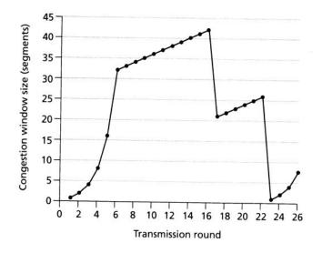
After the 22nd transmission round, is segment loss detected by a triple duplicate ACK or by a timeout event?
