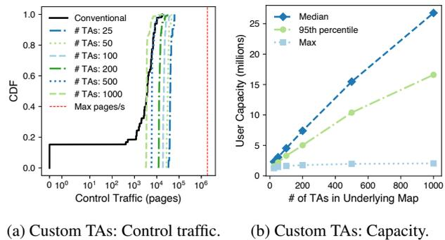
Figure 7: Control traffic and system capacities with custom tracking areas in the simulated environment.
